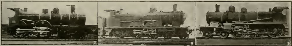
FIG. 7. FOUR CYLINDER, FOUR-COUPLED EXPRESS LOCOMOTIVE OF THE MIDI 1896. FIG. 8. FOUR-CYLINDER COMPOUND ATLANTIC LOCOMOTIVE OF THE NORD, 1900. FIG. 9. TEN-WHEELED EXPRESS LOCOMOTIVE OF THE OUEST RAILWAY, 1901.
